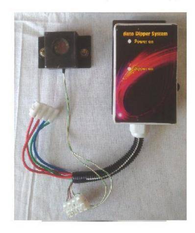
In order to avoid glare of approaching vehicle from front with high beam, the driver (of both vehicles) is required to dip light of his vehicle. At present, this is being done manually with the help of dipper switch. If driver fails to operate dipper switch, driver of other vehicle may not able to see approaching vehicle and may cause accident.
